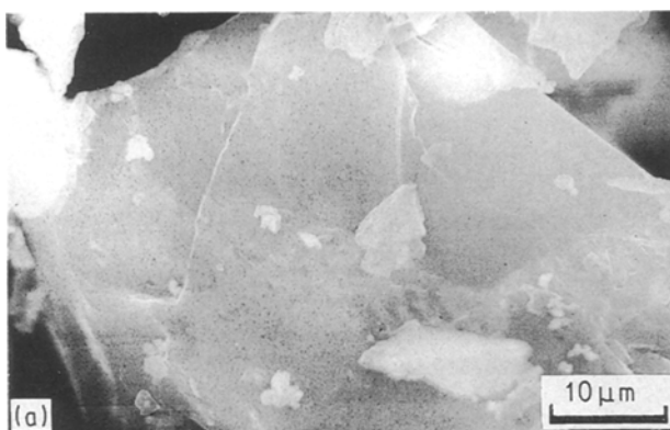
Figure 4 Scanning electron micrographs of the as-synthesized composite alloys (a) \text{La}_2\text{Mg}_{17} -10 wt % \text{LaNi}_5 and (b) \text{La}_2\text{Mg}_{17} -40 wt % \text{LaNi}_5 .
